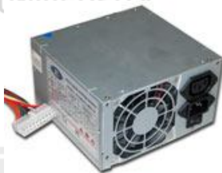
Fig. 1.17: Power Supply Unit
