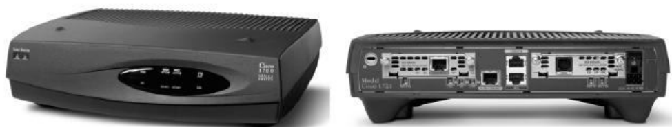
Fig. 2.15: A Common Router with its Front and Back View
